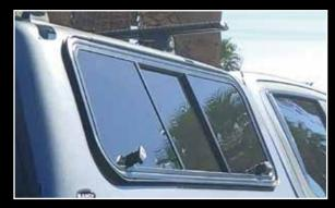
Optional side Windoor with Slider provides ventilation without opening the entire Windoor
